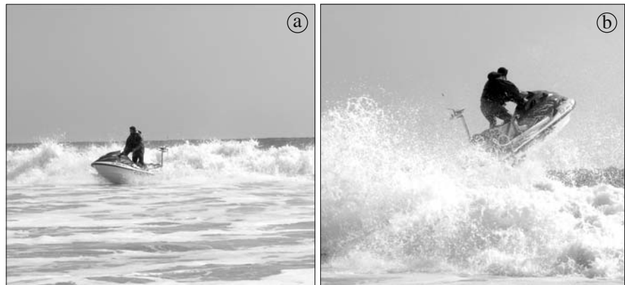
Fig. 10 a Inbound and b outbound cross-shore transects through the surfzone with the jet-ski-mounted WS. a Inbound transect bubbles are minimized by driving just in front of a shoreward-traveling bore. b On outbound transects, bubbly water is drawn into the flow-through WS system as the jet ski drives over a bore
