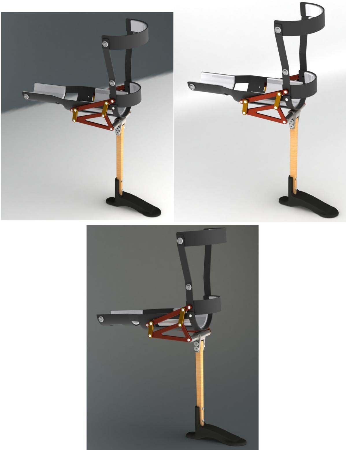
Figure 3.9: Solid model of the fabricated four-bar linkage.
