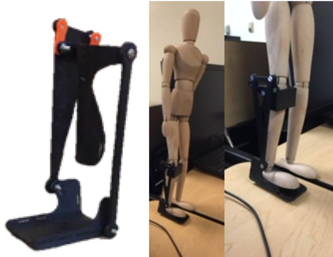
Figure 4.15: Reduced scale 3D printed model of the orthotic device.
