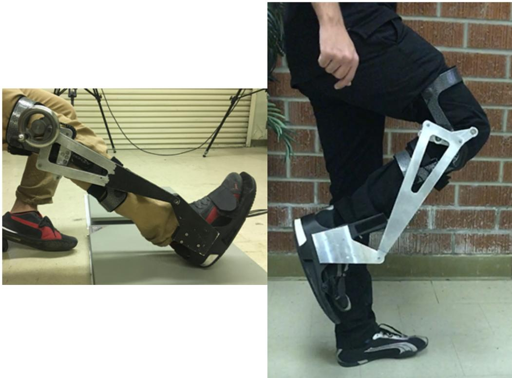
Figure 4.16: Full scale prototype of the KAFO device.
