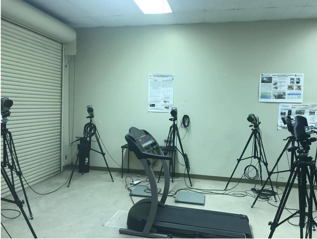
Figure 1.18: Experimental set up for motion capture data collection for locomotion.
