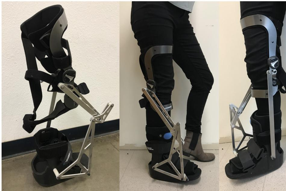
Figure 5.15: Prototype of the new KAFO device.
