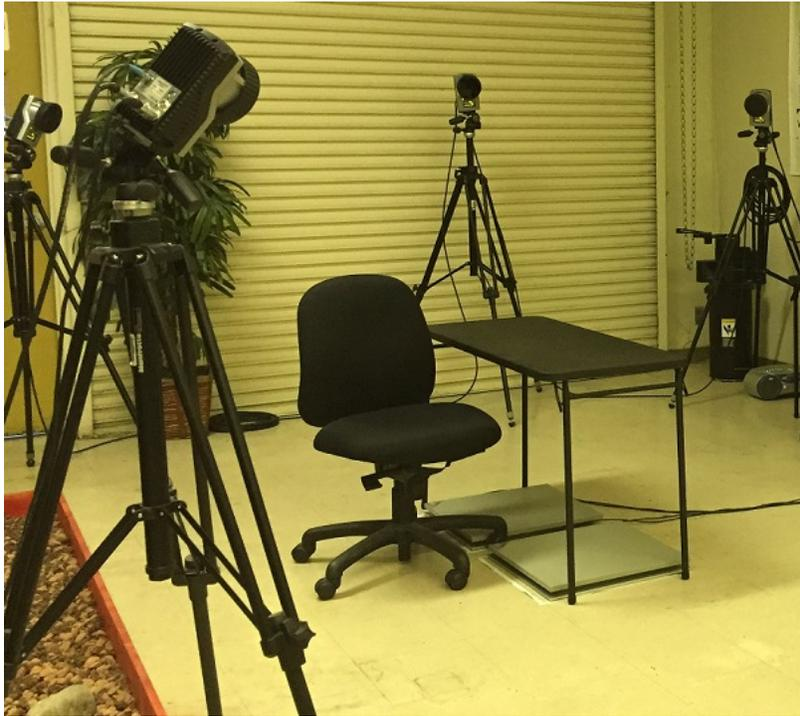
Figure 1.14: The experimental setup showing the capture space and four of the seven Qualisys *OQUS500+* cameras used for motion capture of hand movement.
