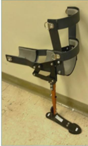
Figure 3.10: Full-scale prototype of the multi-axis hands free crutch.
