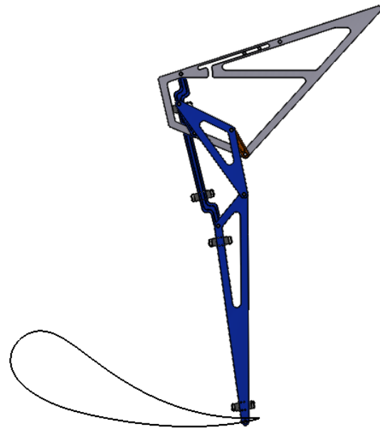
Fig. 11: Solidworks model of the optimized linkage solution
