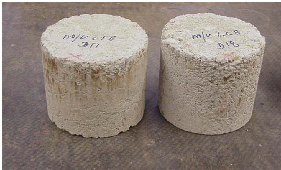
Figure 8. Machine brushed specimens of Mission Valley CTB (left) and LCB (right) materials compacted at Modified AASHTO effort.
