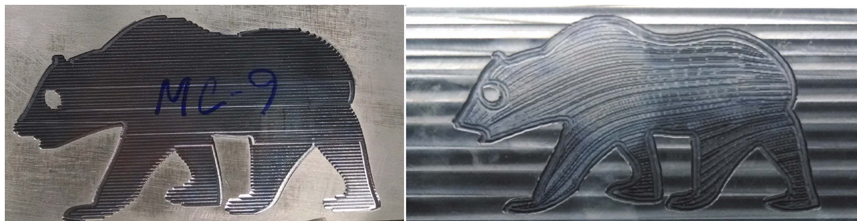
Figure 6.6: Schematic toolpaths for the bear component: (left) using direction-parallel strategy in MasterCAM and (right) using the streamlines generated in digital micrography research.
