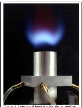
Figure 1 Low-swirl burner with air jet swirler
