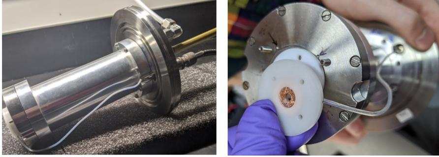
Figure 6.3: Piezoelectric pulsed valve (left) and discharge stack (right).
