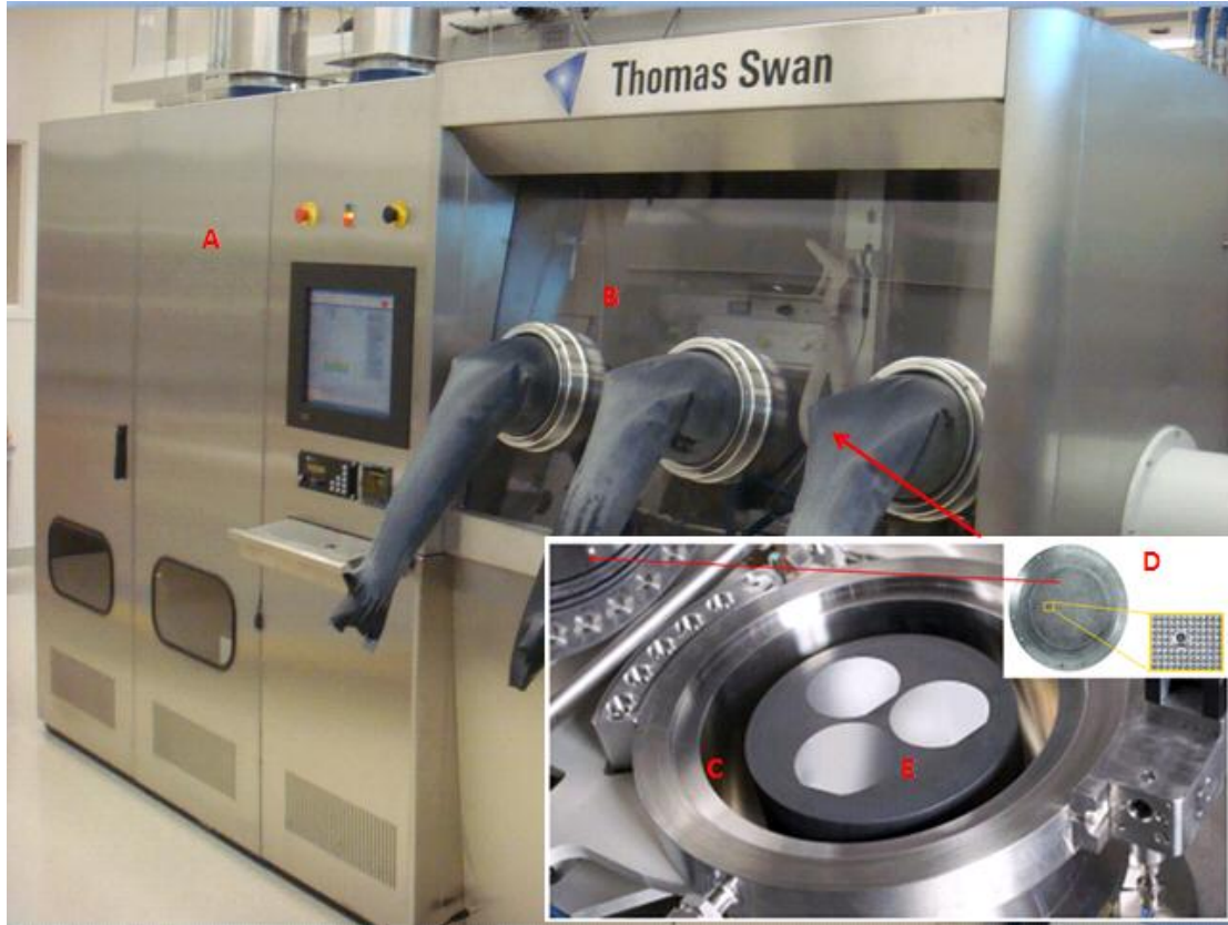
Figure 3-13 Thomas Swan close-coupled showerhead (CCS) 3×2'' MOCVD system. A: Metal-organic sources cabinet; B: Glove box; C: Reactor chamber; D: Showerhead; E: Susceptor.
