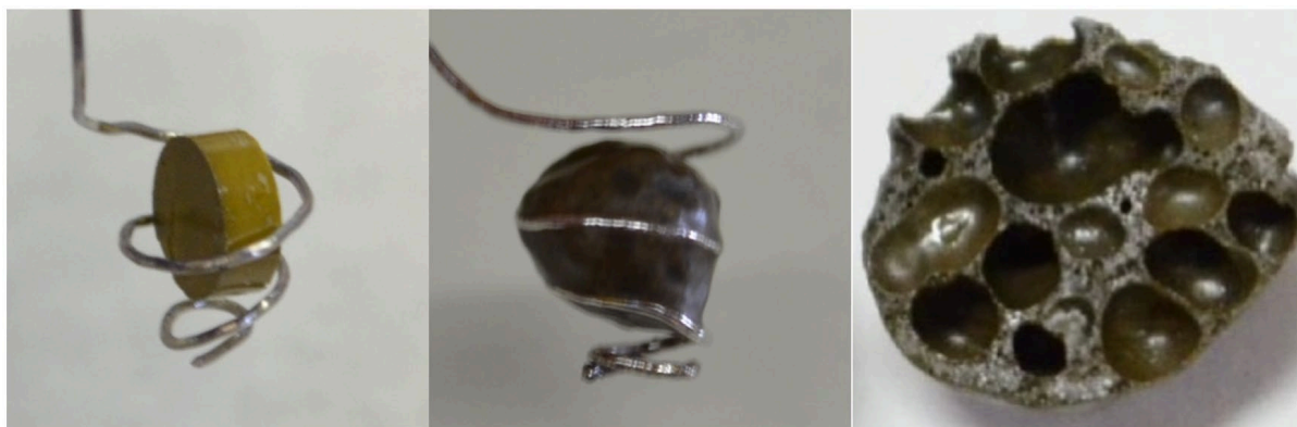
Fig. 7.3: Illustration of the coiled wire design to support samples that melted substantially without climb or dripping out of the container. The porous structure of the sectioned sample suggests gas evolution during the partial reduction of \text{Fe}^{3+} to \text{Fe}^{2+} .
