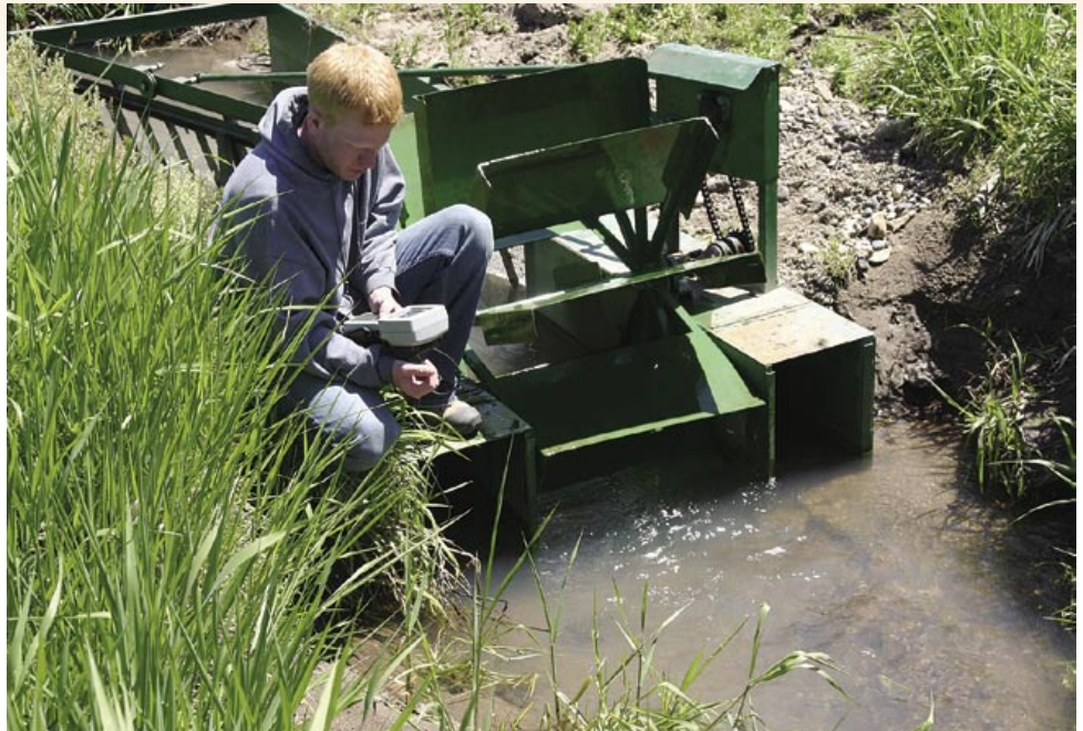
Irrigated pasture provides critical summer forage for California livestock, but the environmental impacts on fish of diverting streams to pastures are coming under increasing regulatory scrutiny. Above, Shannon Cler, UC Davis postgraduate researcher, measures dissolved oxygen in a delivery ditch in lower Lassen Creek.
