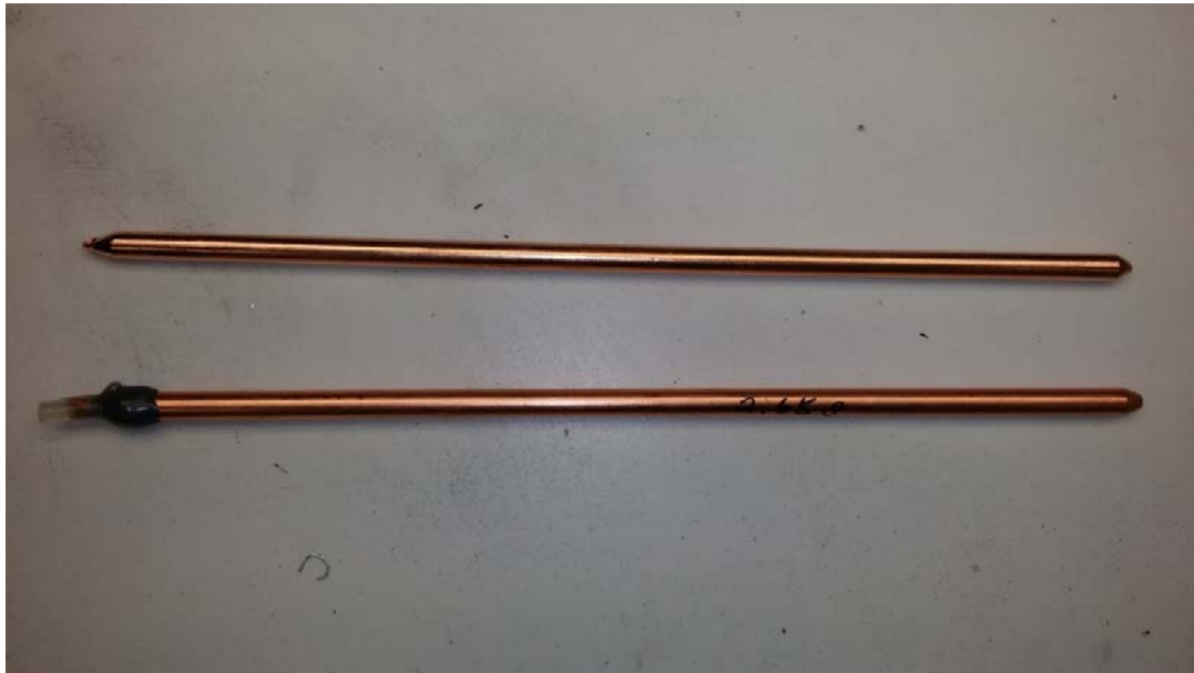
Figure 105: Original Enertron heat pipe and recharged heat pipe
