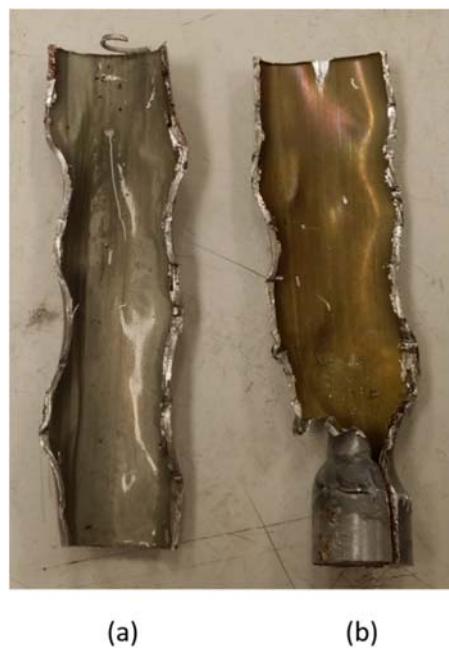
Figure 111: Cut open aluminum/IAS thermo-syphon: (a) condensing region; (b) evaporating region
