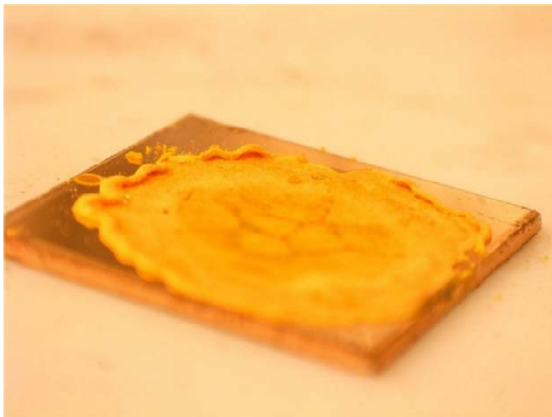
Figure 77: Sample surface coated by potassium chromate in the coating study test
