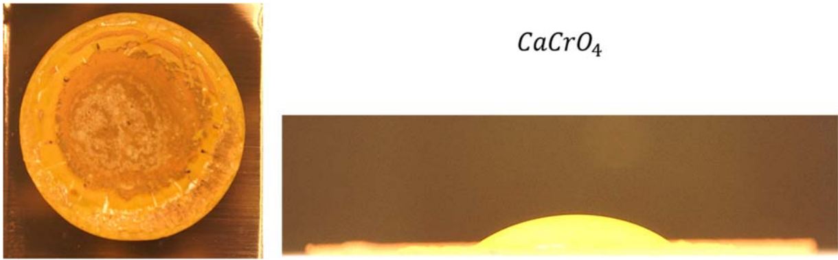
Figure 50: DI-water on mirror like copper surface cooked by calcium chromate
