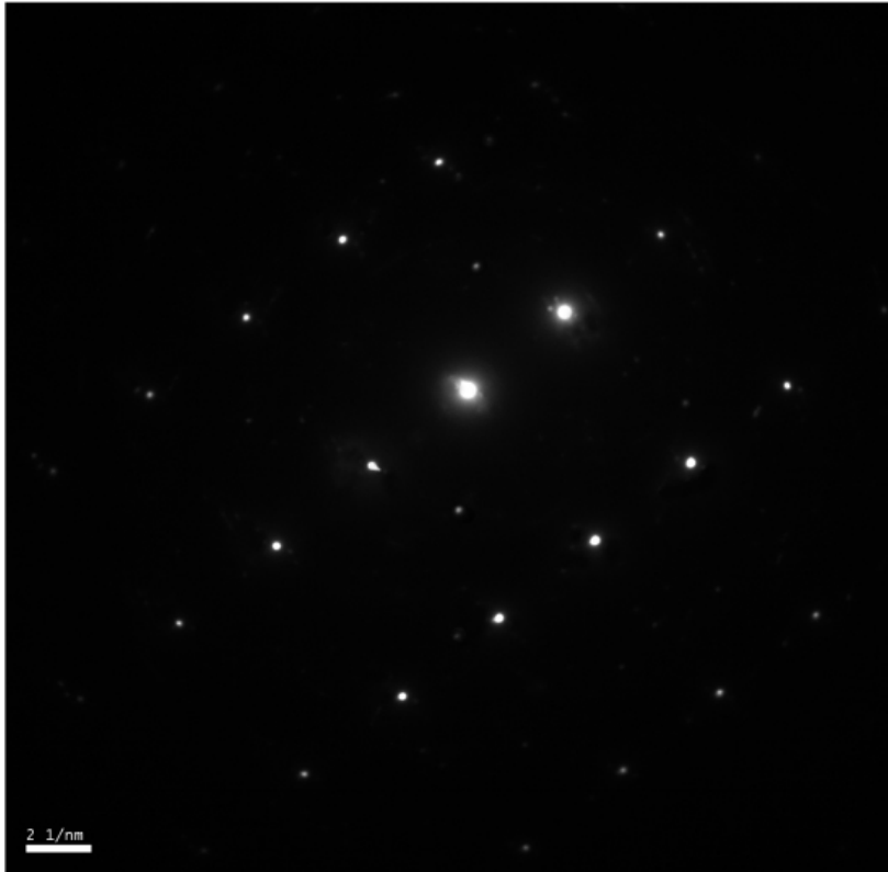
Figure 4.13 The nanopillar after compression, bright field image and diffraction pattern; only grain “A” and grain “C” can be seen. Grain “B” disappeared. BD=[2-1-10] .
