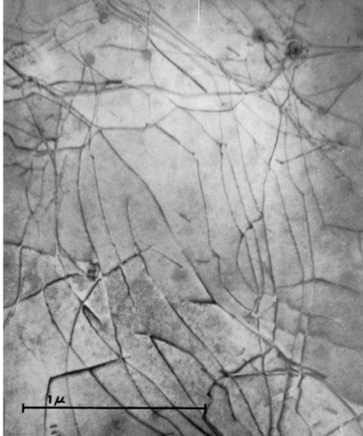
Figure 1.9. Basal dislocations in a 45-degree compression specimen. ~5% Strain. (R.T. Tsui, 1967)(31). Large number of basal dislocations can be usually observed in the deformed microstructure.
