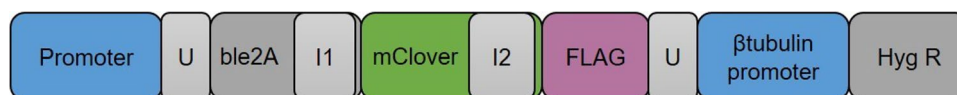
Fig. 1 Design of double-antibiotic resistance expression vector. The variable “Promoter” region is upstream of the rbc2 5' and 3' UTRs (U). The ble2A gene for zeocin resistance is fused to an mClover
