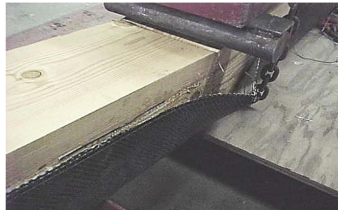
Fig. 13. Failure of Group “A” retrofitted beam specimen.
