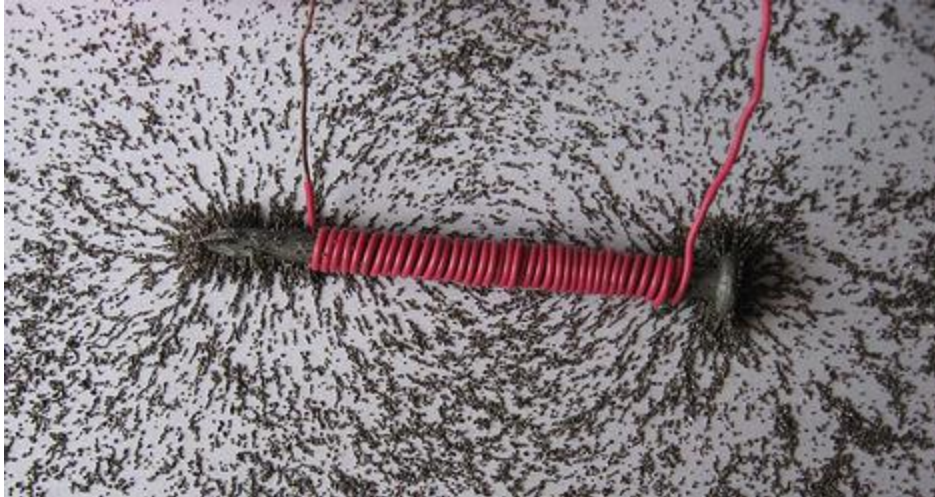
Figure 1.1 - An iron nail wrapped with a current carrying wire aligns surrounding ferromagnetic iron filings to equipotential magnetic field lines [Google Images]
