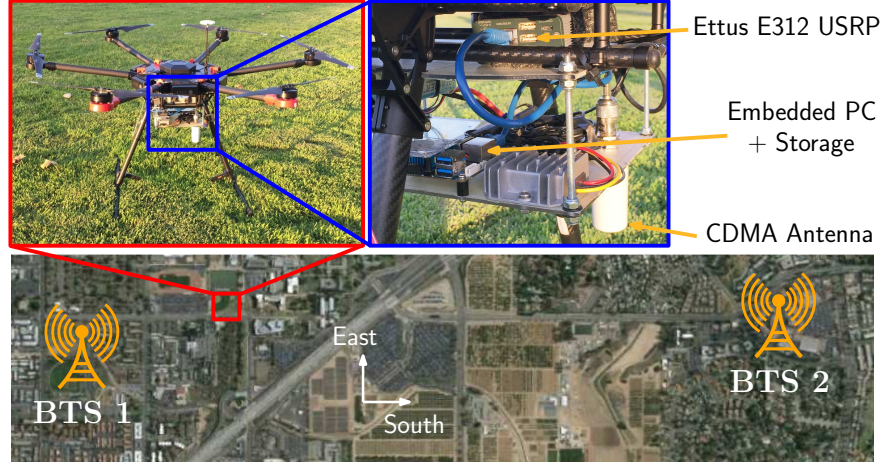
Figure 2.13: SOP BTS environment and experimental hardware setup for the UAV experiment. Map data: Google Earth.
