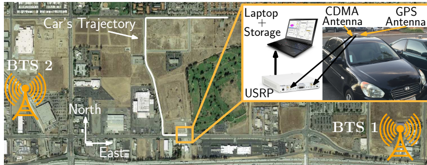
Figure 2.16: SOP BTS environment, true trajectory, and experimental hardware setup for the ground vehicle experiment. Map data: Google Earth.
