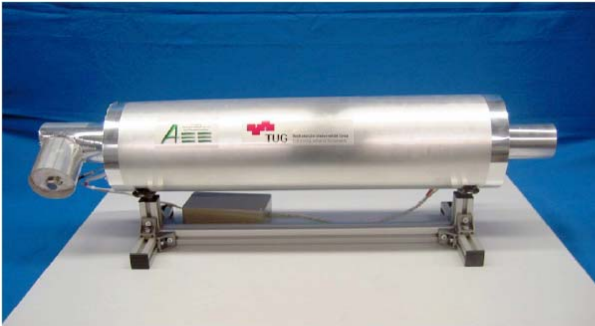
Figure 4: Third Generation AES ammonia cracking unit developed at the Technical University Graz (Source: Aronsson, 2007)
