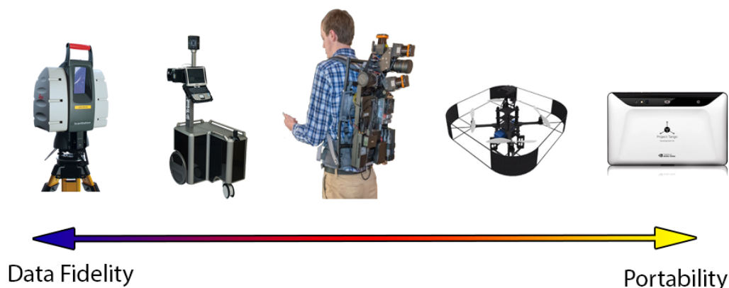
Figure 1.1: The spectrum of indoor mapping solutions. The existing solutions can be viewed as a trade-off between portability and data fidelity. In one extreme, static scanning solutions provide the highest quality data but are slow and cumbersome to use. On the other end of the spectrum, R-GBD depth cameras are small and mobile, but often contain noisy sensing technologies.
