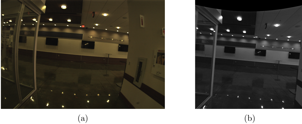
Figure 2.3: An example of applying image undistortion to a fisheye image. (a): The input distorted fisheye image. (b): An undistorted version of a subsection of the input fisheye image.
