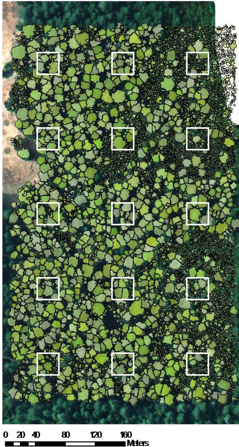
Figure 3-7. The result of individual tree detection and delineation by the proposed method. White squares represent the reference plots used for accuracy assessment.
