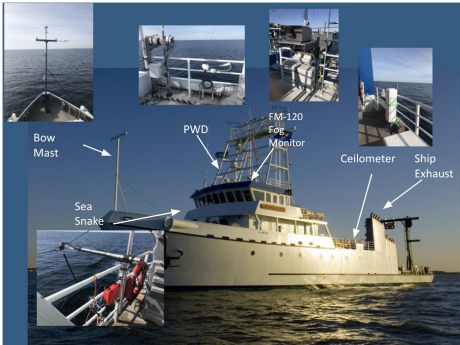
Fig. 2 Instrument positions on-board the R/V Hugh R. Sharp and pictures of key instruments taken during the campaign relevant to the present study. Adapted from Fernando et al. (2020)
