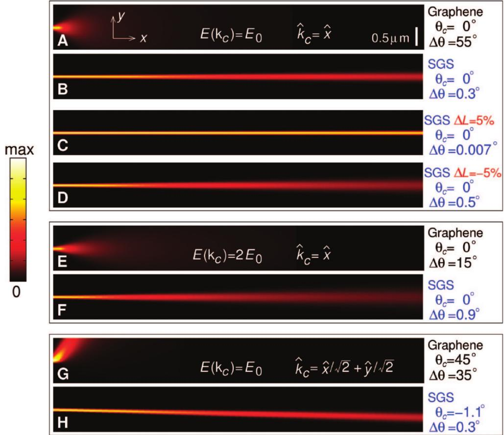
Figure 3.3: Graphene under 1D periodic potentials as an electron supercollimator. [10]. In this figure, one can see how electrons propagate in graphene and in graphene under periodic potentials with differing conditions.
