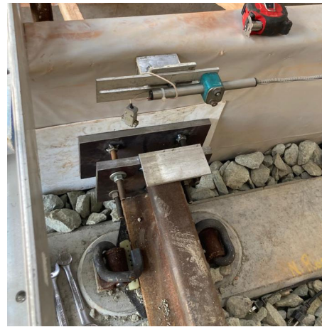
Figure 6. Instrumentation layout: (a) Plan of representative section, and (b) Constructed rail embankment after instrumental placement; (c) Rail-wall connection detail.
