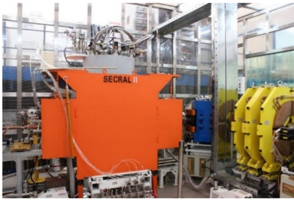
FIG. 3. SECRAL-II ECR ion source at beam commissioning.
