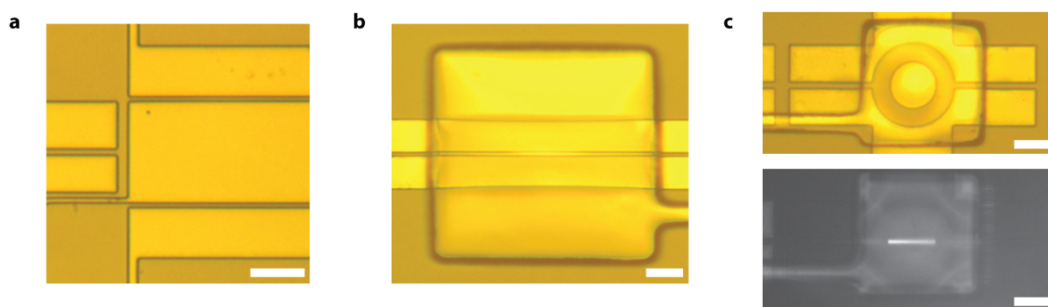
Fig. 7.8 | Example PDMS Waveguide Platform Microscope Images. a , Reconfigurable optofluidic MMI, empty, b , Lightvalve in its static state, empty, and c , Lightvalve trap, both empty (top) and filled and under optical excitation (bottom). The filling fluid for the lightvalve trap is a 3 \mu\text{M} Dylight 488 solution and exhibits fluorescence when excited by 488 nm laser light, injected from the left solid-core waveguide. Note: all white scale bars represent 50 \mu\text{m} .
