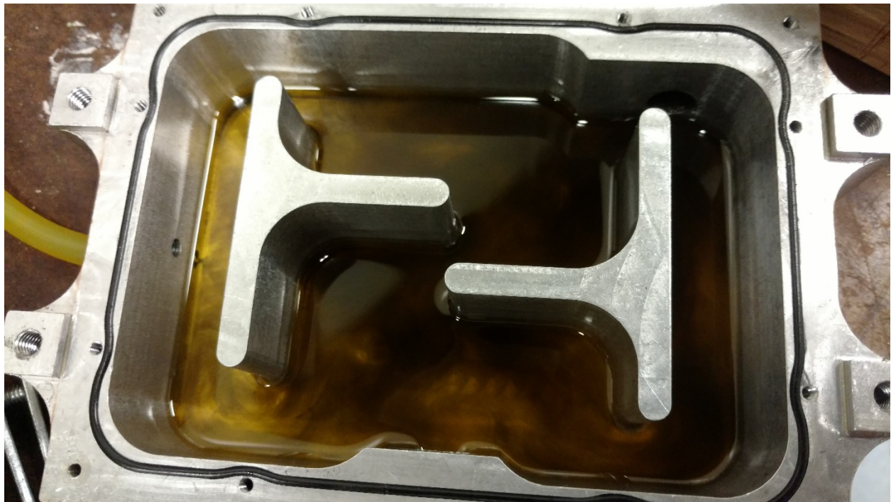
Figure 71: Image showing fine particulate matter in the oil reservoir of the flywheel
