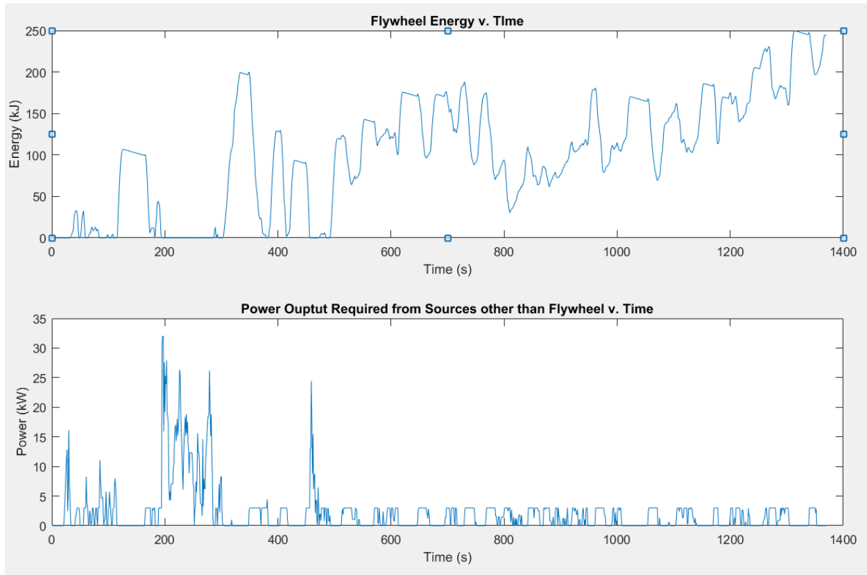
Figure 39: Plots showing flywheel energy (top) and power required from sources other than battery (bottom) for a driving strategy attempting to minimize discharge peaks while sacrificing a small amount of efficiency.
