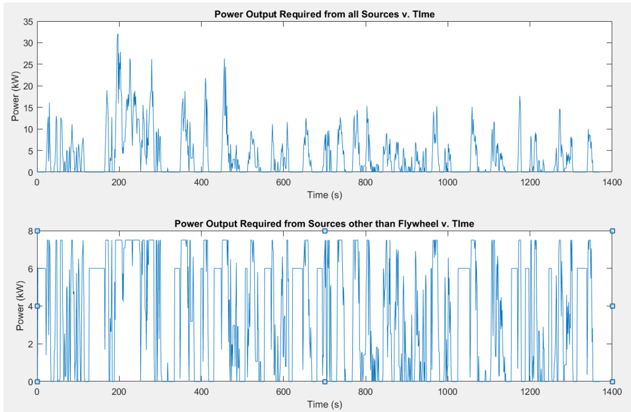
Figure 43: Total power required to complete driving cycle (top) and power required from sources other than the flywheel (bottom) for a driving strategy involving a 6 kW pre-charge of the flywheel, and a 7.5 kW power output of the ICE/battery combination.
