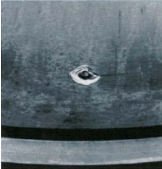
Figure 78: Electrical pitting corrosion on the race of a ball bearing. [34]
