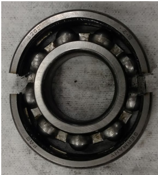
Figure 73: Bearing cut to gain access to races and bearings
