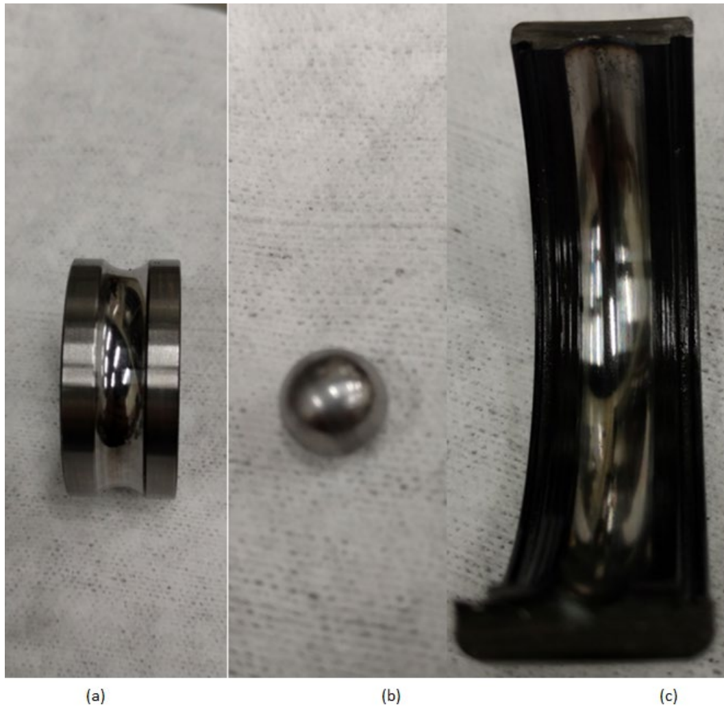
Figure 74: View of inner races of bottom bearing. (a) Inner race (b) ball (c) outer race.
