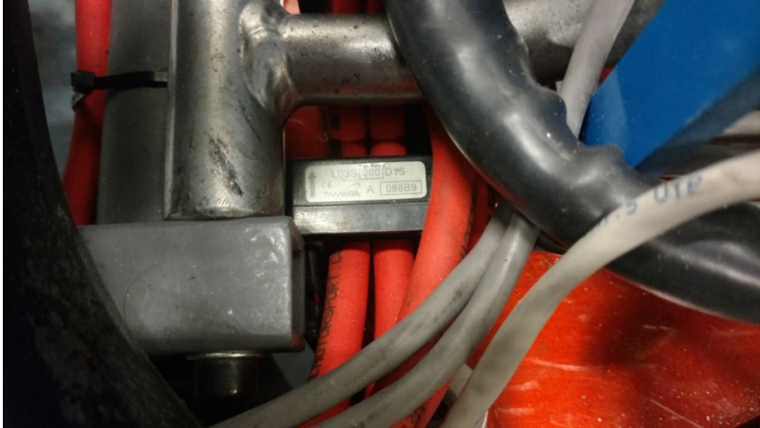
Figure 11: Temura Hall Effect Current Sensor. The sensor in this image is the black rectangle surrounding the two orange power cables. There is one cable for each battery pack.
