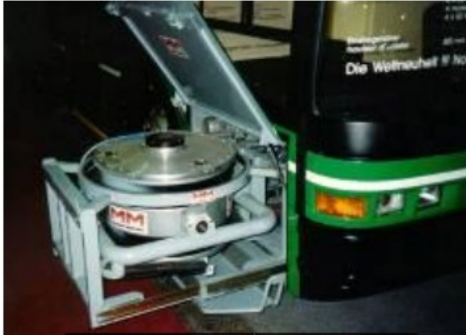
Figure 8: L-3 Communications Magnet-Motor GmbH fitted to an urban hybrid bus [11]
