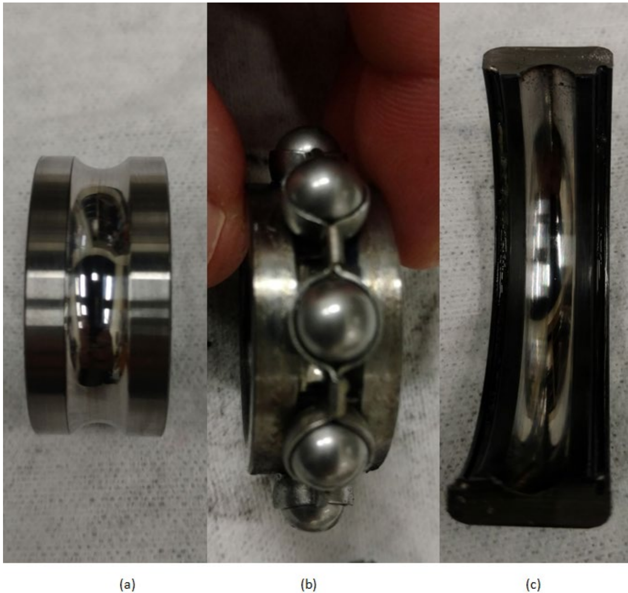
Figure 75: View of races of top bearing. (a) Inner race (b) ball (c) outer race.
