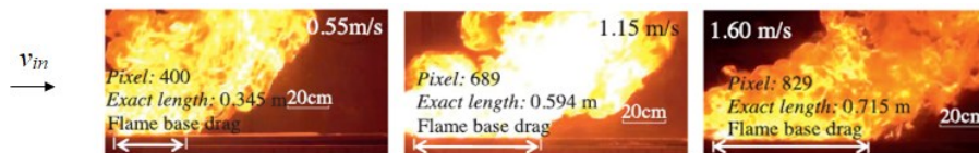
Fig.1 Flame images at different longitudinal air velocities for a 60cm heptane pool fire (Hu, L. et al.,2016)
