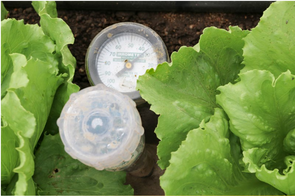
Figure 4. Monitoring soil moisture with a tensiometer can help growers decide when to irrigate. Tensiometers measure the energy that plants require to uptake water from soil. High tension values in units of kilopascals or centibars indicate dry soil conditions. Photo: M. Cahn.
