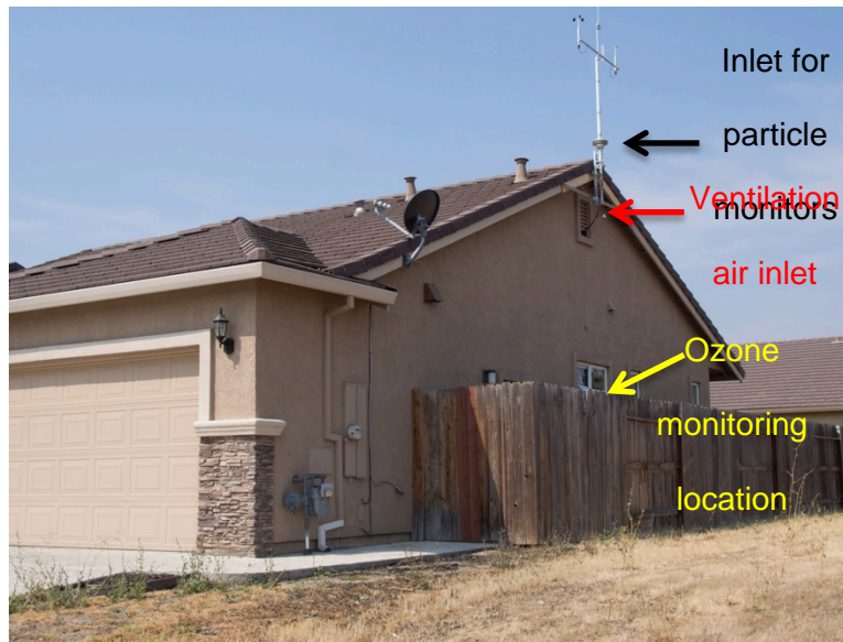
Figure S.8. Weather station and air intakes for supply ventilation and outdoor particle sampling.
