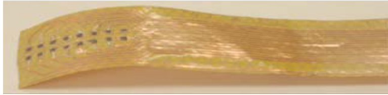
Figure 3.1: A 16-element conformal ultrasound array prototype of which one 1 \times 8 row was tested.
