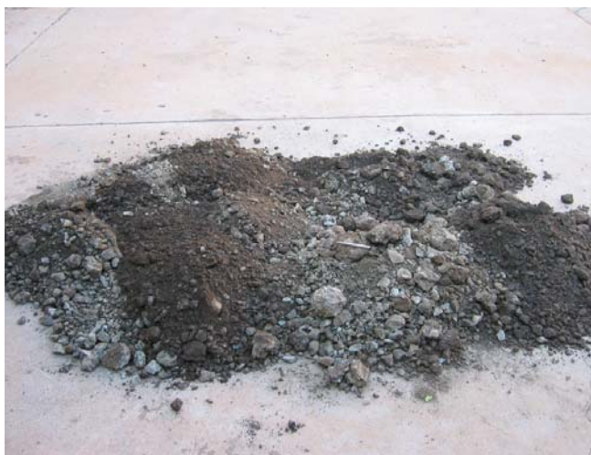
Figure 3.13: Base course material from test pit. (Note large cemented lumps.)
