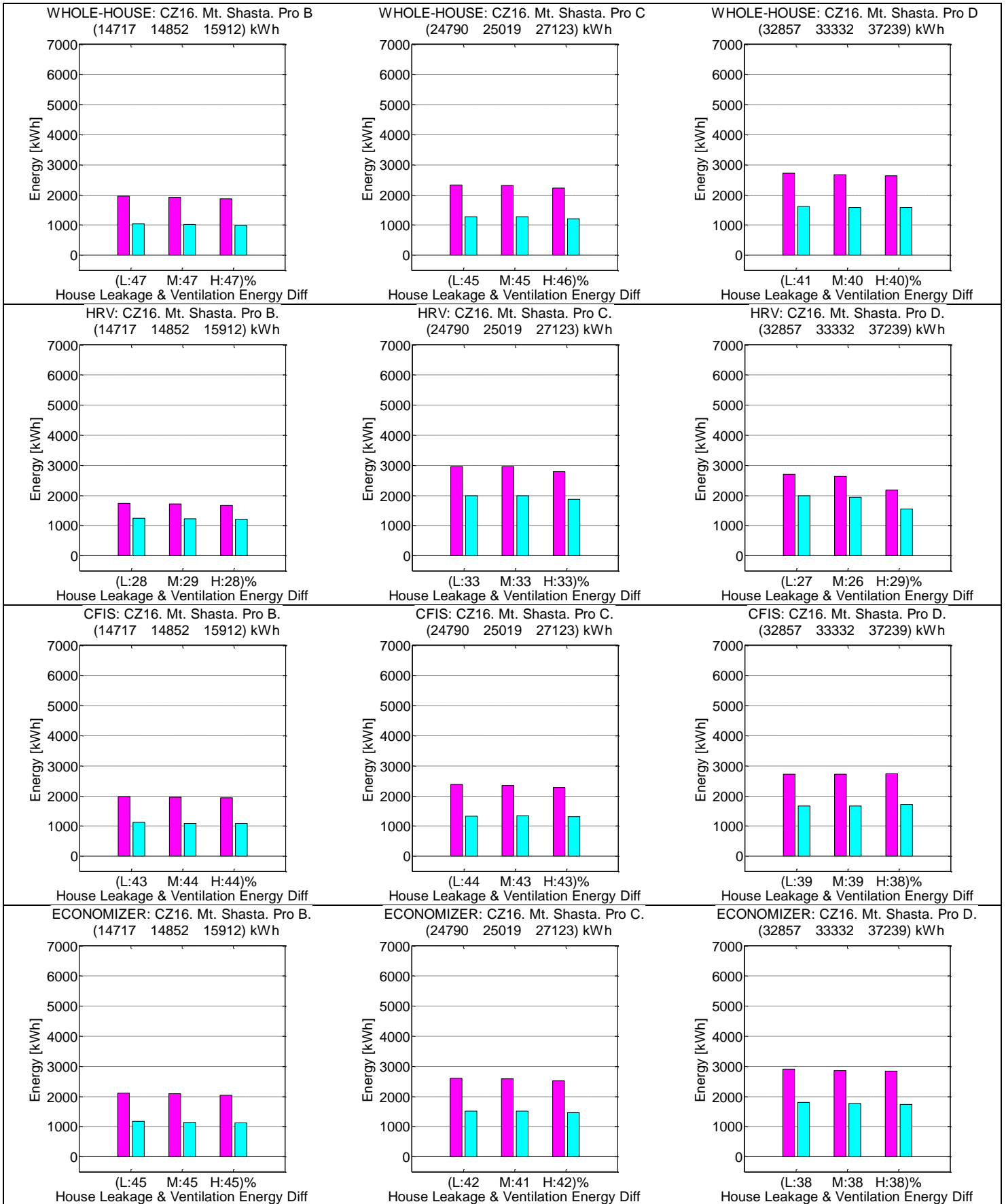
Figure 44: Ventilation-related energy penalty with and without RIVEC for climate zone 16, Mount Shasta
