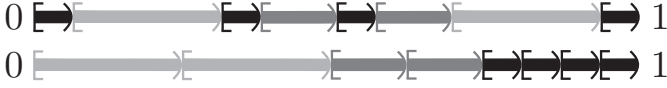
Fig. 2. Two optimal quantizers for the unit interval [0, 1] when r = 2 . Each quantization cell is a half-open interval. Length- \frac{1}{4} light gray intervals, length- \frac{1}{8} dark gray intervals and length- \frac{1}{16} black intervals are the quantization cells for reproduction points whose indices have weights 4, 16, and 64, respectively. The reproduction point for any given interval is located at its center.
