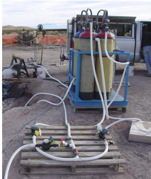
Figure 4-3. Flowing fluid electrical conductivity log performed in 420 meter open borehole in the Amargosa Valley, Nevada.
