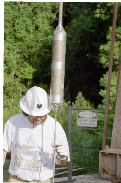
Figure 4-1. Installation of an orbital vibrator borehole seismic source used for cross-well seismic surveys in east Texas, USA.
