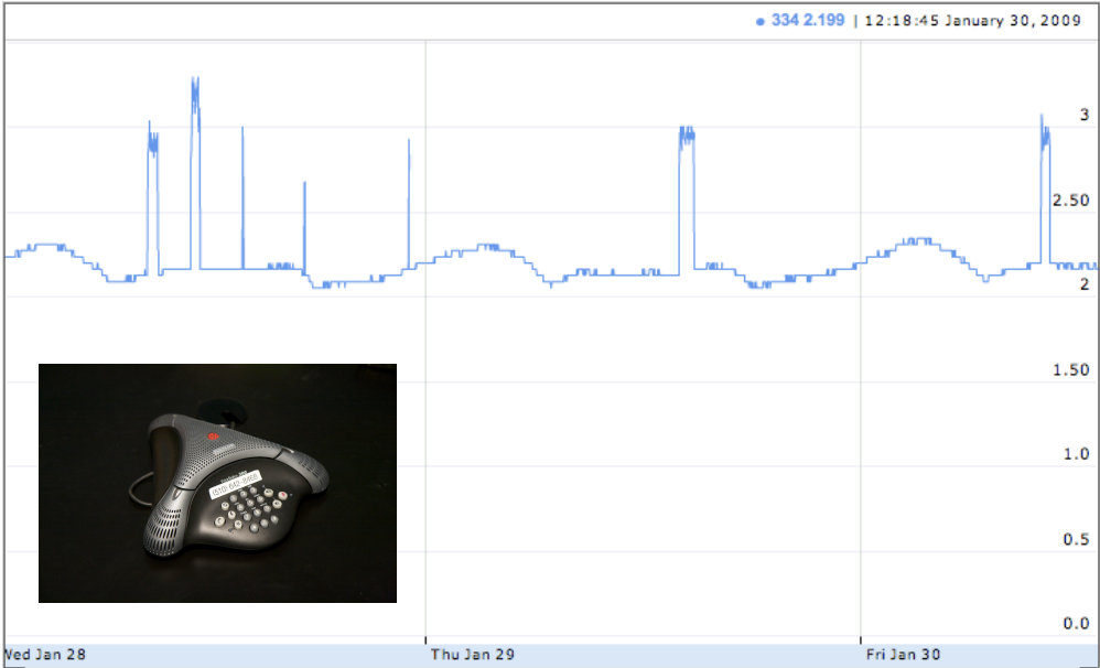
Figure 4.6: Power trace of a Polycomm telephone shows that ACme-A is able to resolve low power appliances down to 40mW.
