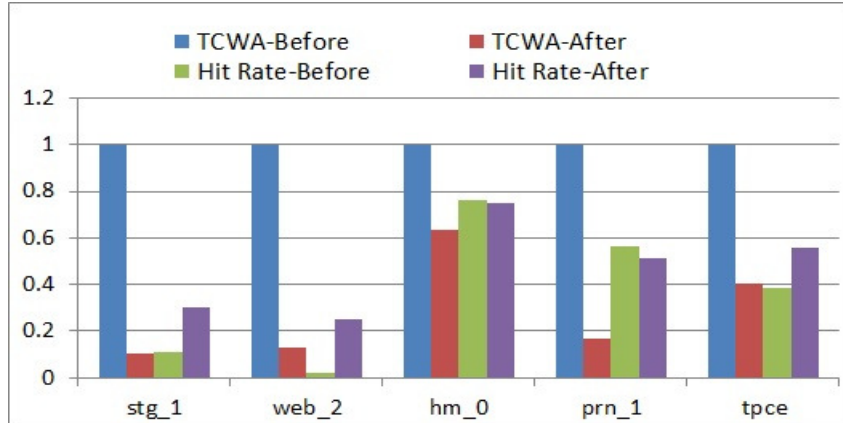
Figure 3.6: Comparison of TCWA and hit rate before and after cache and flash layer optimizations: TCWA is significantly reduced with well-selected algorithms. Hit rate maintains a certain level and is improved under some workloads.
