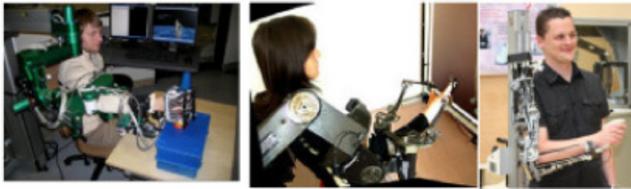
Figure 2 Example upper extremity exoskeletons with at least four degrees of freedom, including ARMI from ETH Zurich (left, 27), the L-Exos from Scuola Superiore Sant'Anna, Pisa, Italy (middle, 28), and the Able Exoskeleton from CEA/ISIR/Haption in France (right, 29).
