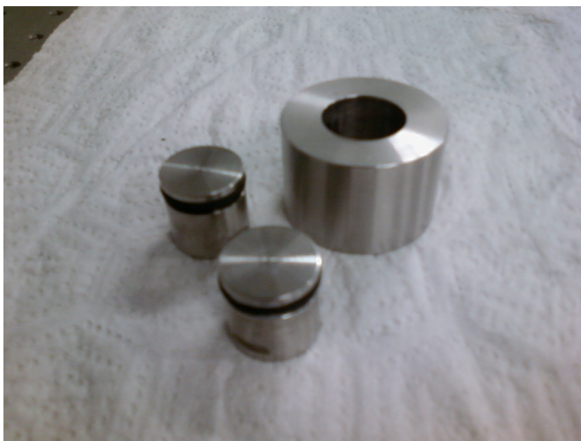
Figure 4.3 – A piston typical of the type used to compress the mixture. Omitted from the picture is a copper sleeve which is inserted around the perimeter to reduce mechanical friction.
