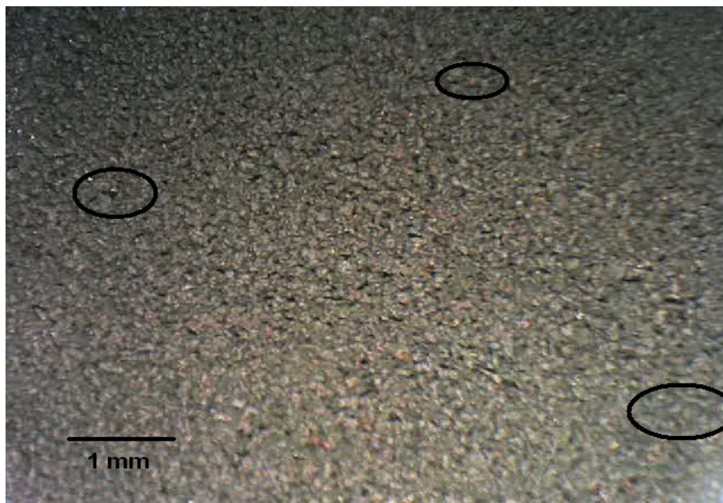
Figure 2.10 – A view of water drops (in black circles) on the surface of a porous monel cylinder, brought from a 0-degree environment. Magnification is 20X.
