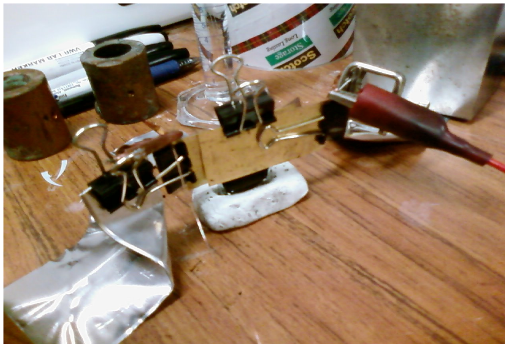
Figure 4.8 – The electrode module with the epoxy mold filled with solution. Copper leads were used to connect the metal plates to the alligator clips.
