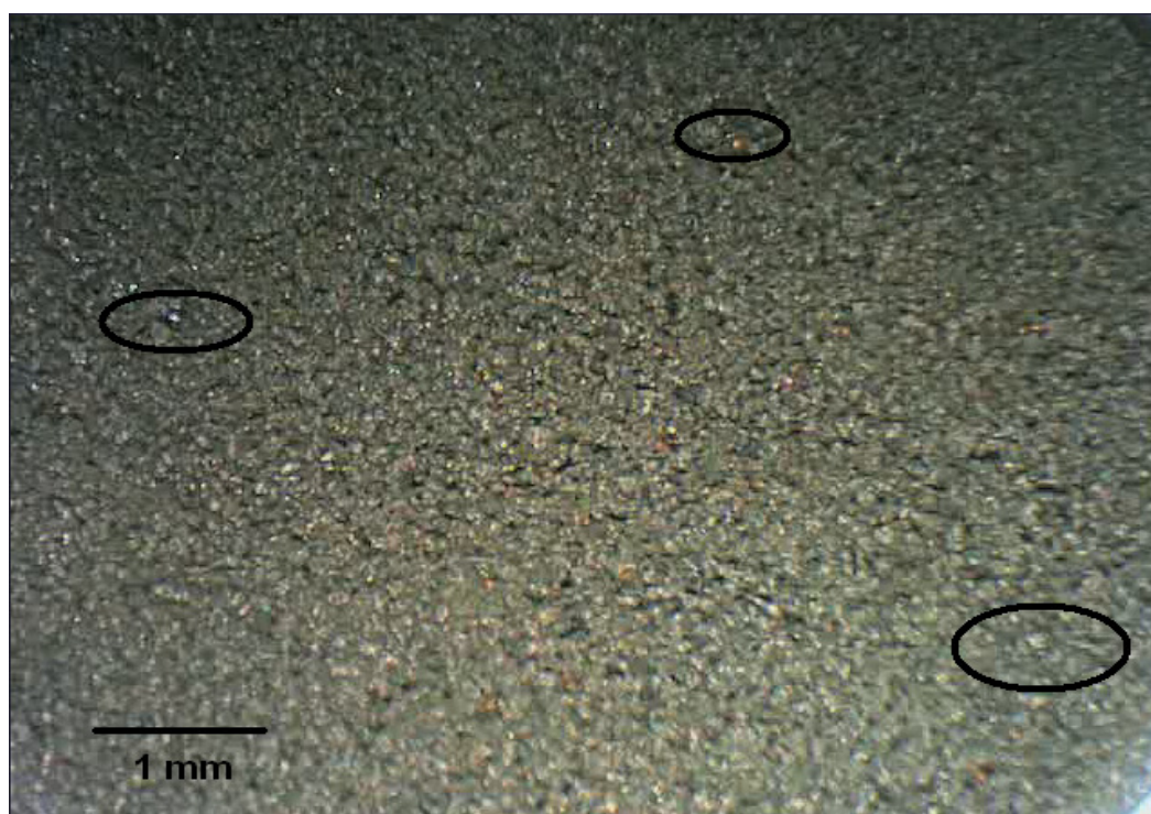
Figure 2.11 – A view of water drops, from the same area on the monel cylinder, taken 3 minutes after Figure 2.10. Magnification is 20X.
