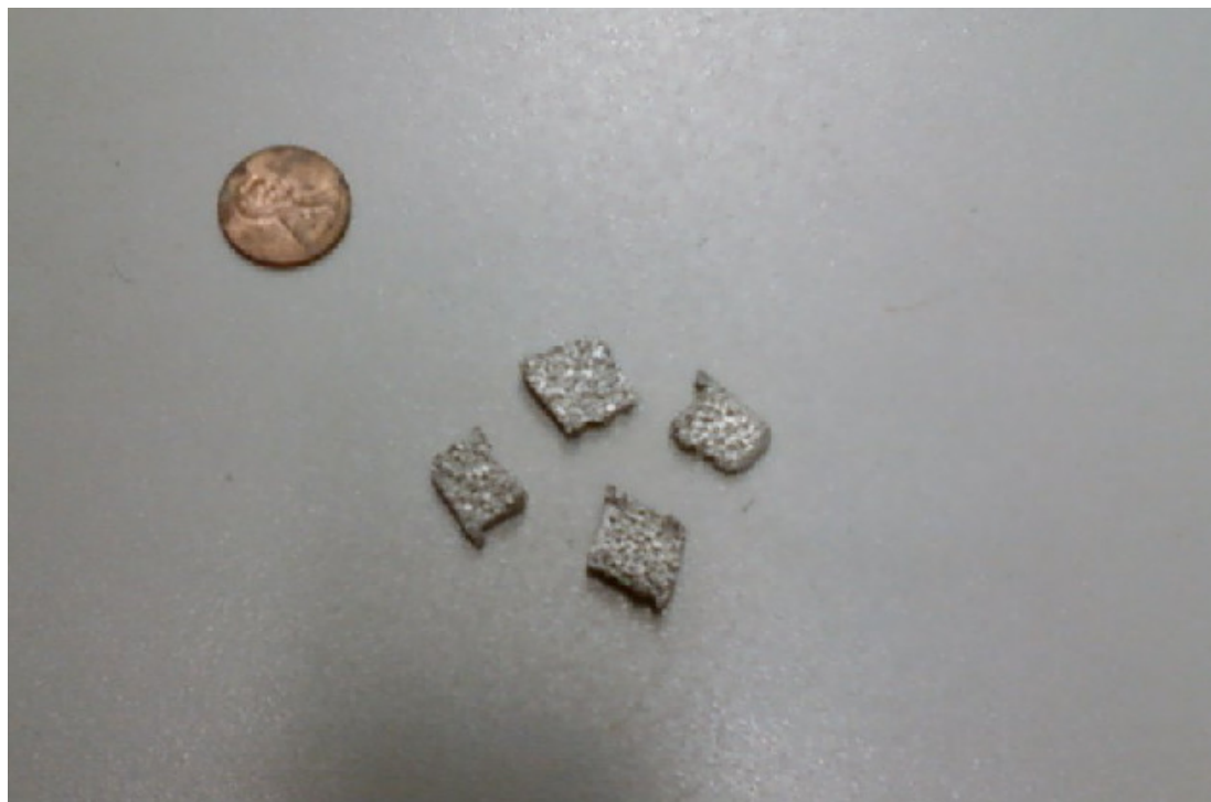
Figure 2.2 – Photo of porous aluminum samples which exhibited hydrophobicity after C8 surface treatment, with a penny shown for scale.
