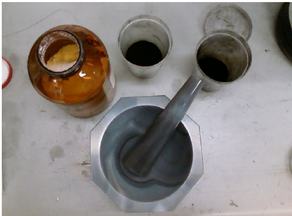
Figure 4.2 – The three ingredients used to produce the electrode, from left to right: PVDF, AB50, and BP2000. The agate mortar and pestle is shown on the bottom.
