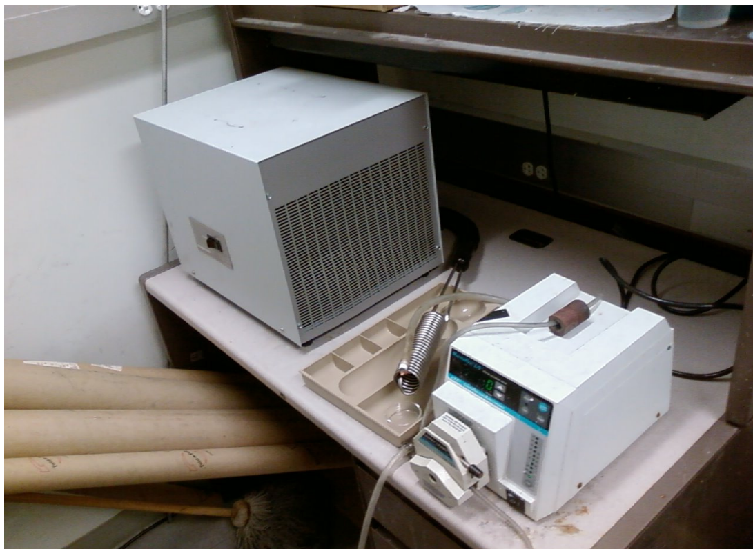
Figure 2.6 – A picture taken of the setup configuration of the immersion chiller, air pump, tube, and monel cylinder.
