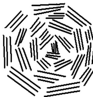
Figure 1.6 – A sketch depicting the simplified model of carbon black based on concept by Heckman and Harling [19]. Under oxidation, the radially positioned layers exfoliate.
