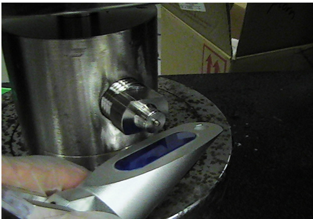
Figure 3.8 – The process of collecting drops for measurement, where the refractometer was positioned directly beneath the tap opening.
