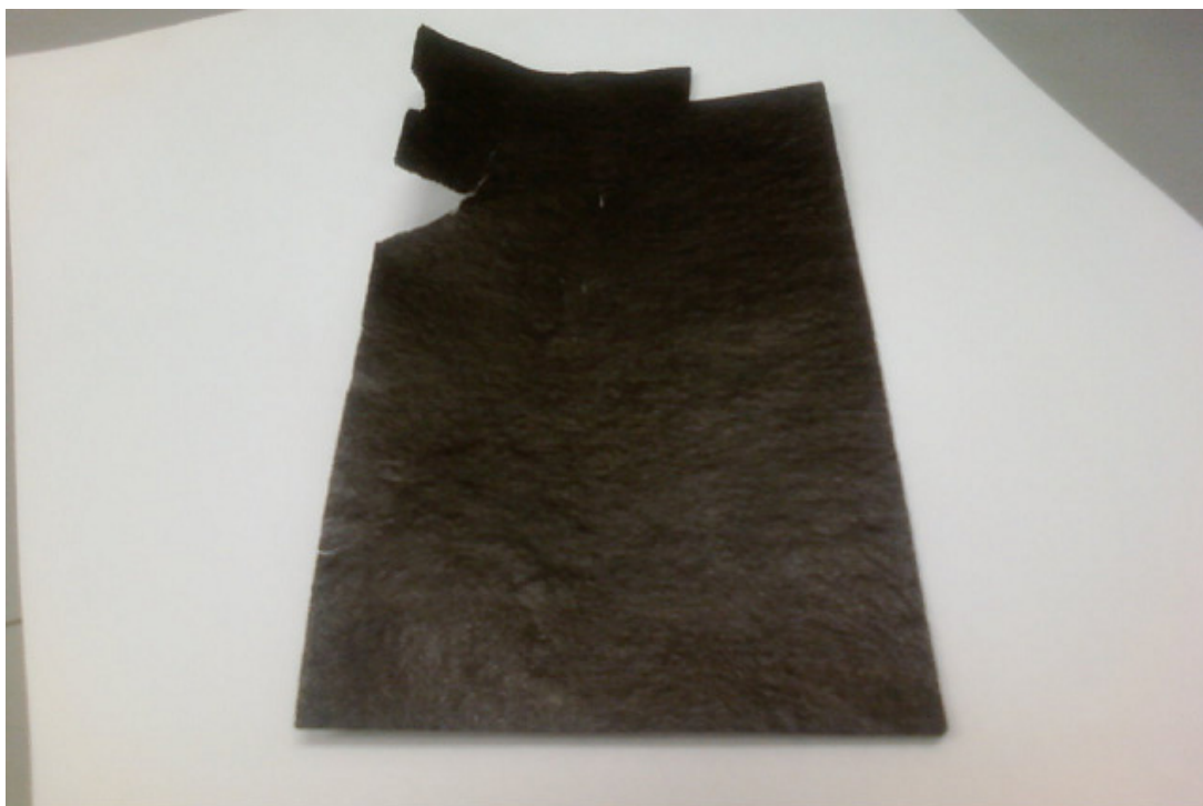
Figure 1.7 – Carbon aerogel sample. The fragile nature is evident by the tear in the upper left corner.
