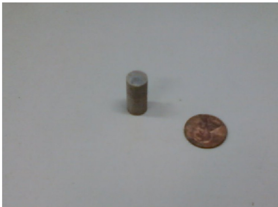
Figure 2.3 – Photo of the monel cylinder, surface treated with C8, with a penny shown for scale.
