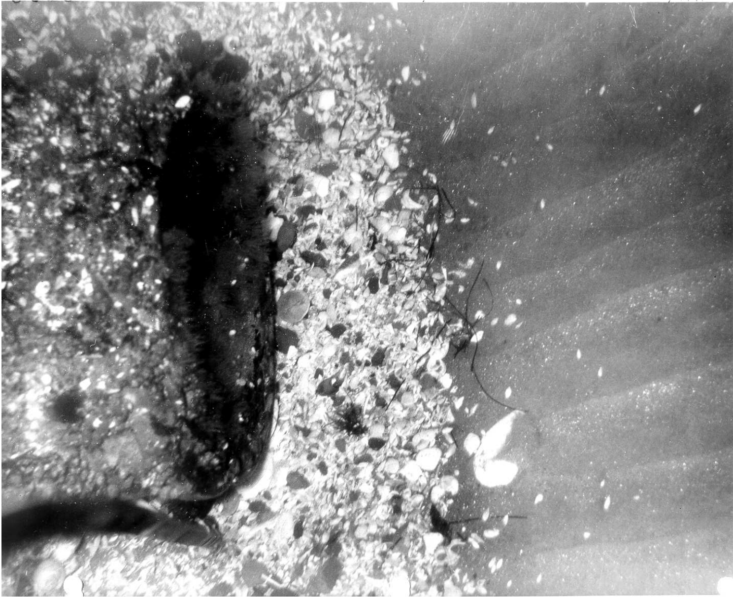
Figure 2-6. HM MARK 36 mine at 17 m depth, 9 months after laying, with major scour depression that has scavenged an aggregate of coarse material. Mine completely buried several days after this photograph. [Inman negative 339-3, Jan 1954]
