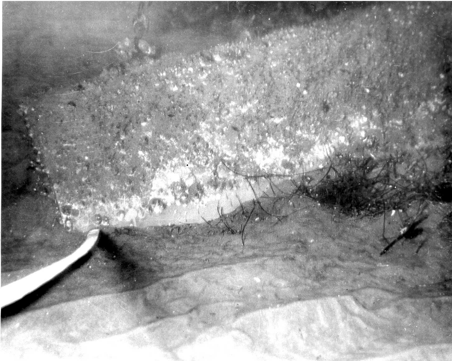
Figure 2-7. HM MARK 36 mine at 23 m depth about three-quarters buried, nine months after laying, just before total burial as shown in Figure 2-8. [Inman negative 343-1, 1954]
