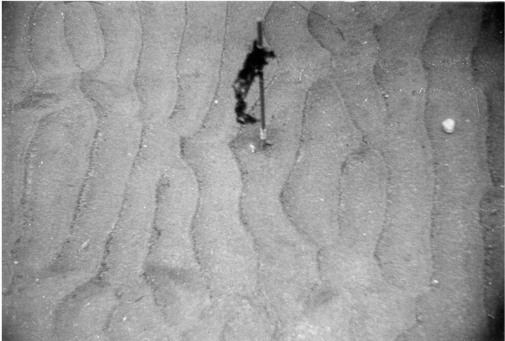
Figure 2-2. Reference rod used to determine sand level change at mine site in depth of 9 meters on the shelf off Scripps. Brass rod is 1 cm diameter and 122 cm long, approximately 30 cm exposed. Ripple wavelength is about 7 cm in sand of median diameter 125 \mu m. [from Inman and Rusnak, 1956]
