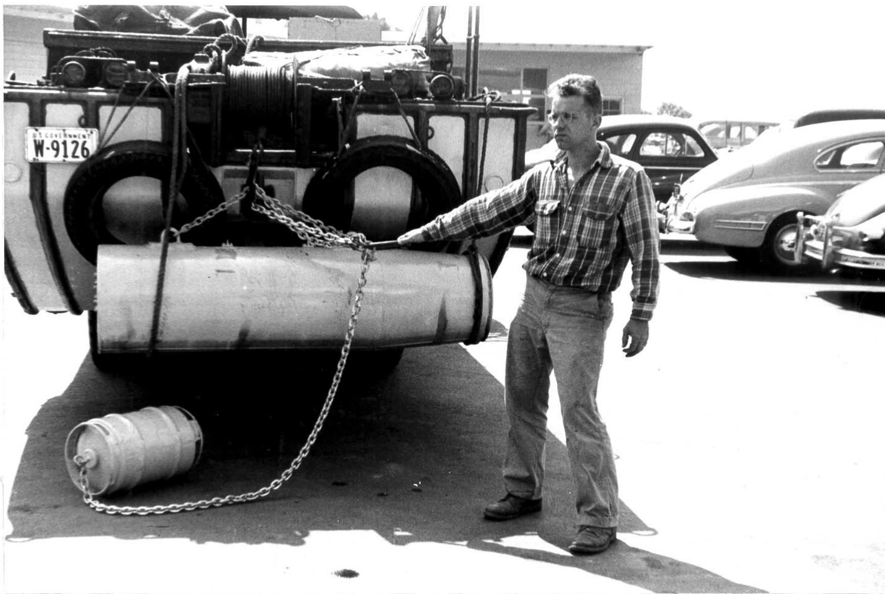
Figure 2-1. HM MARK 36 mine on stern winch of a DUKW in preparation for deployment off Scripps in 1953. The subsurface buoy is to aid in location on the seafloor. [from Inman and Jenkins, 1996]
