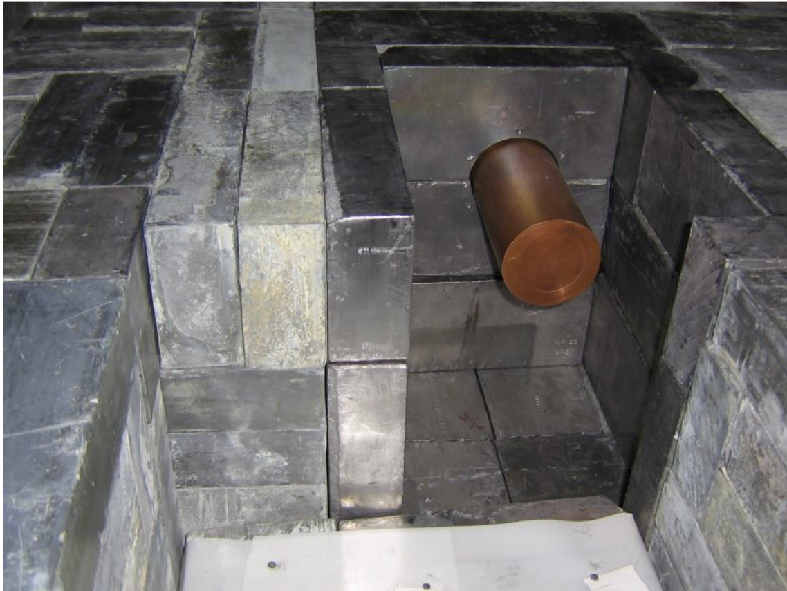
Figure 2: The open SOLO chamber. The 0.6 kg high-purity germanium detector is housed in a 1.5 mm thick copper shield. The chamber is lined with >30 cm of lead shielding. The inner 5 cm lead layer was selected for its measured ^{210}\text{Pb} content (<50 mBq/kg).
