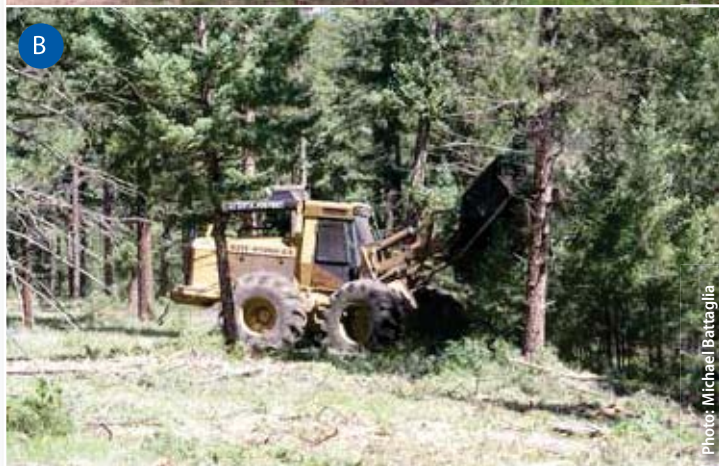
Figure 12. Mastication heads can be mounted on wheeled and tracked machinery. Many styles are available for treating brush and small trees. A masticator head is mounted on a wheeled skidder (A). The masticator head is being lowered onto small trees to shred them (B).
