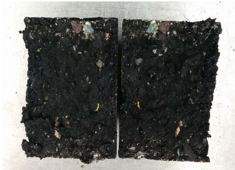
Figure 2.19 Post-test IDT specimen exhibiting fractured aggregate.
