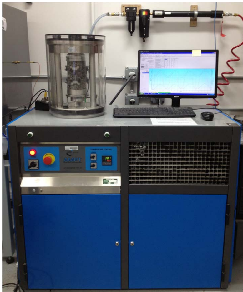
Figure 2.11: AMPT testing setup for HMA dynamic modulus with axial LVDTs mounted on the specimen.
