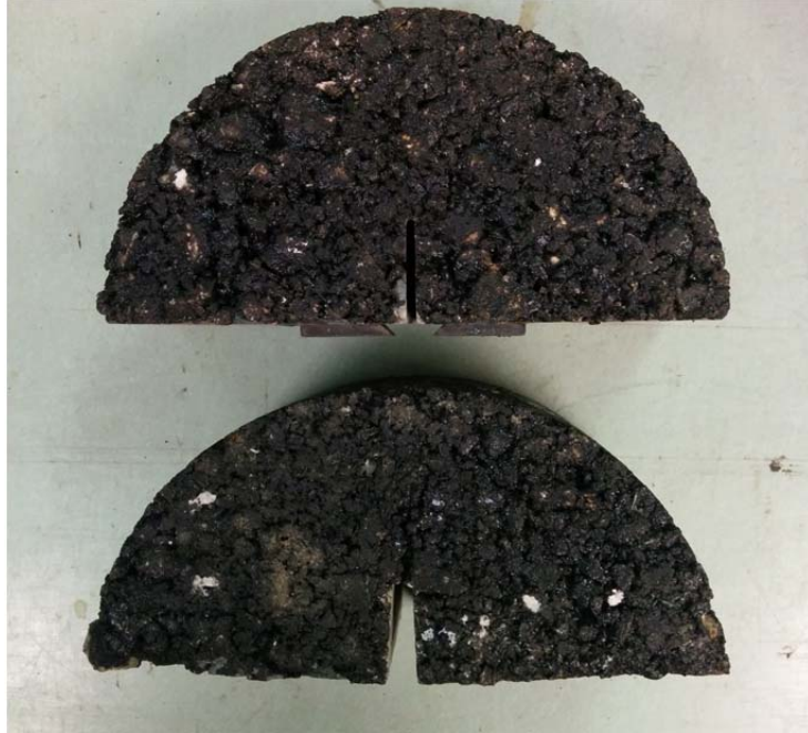
Figure 2.21: Semicircular beam (SCB) specimens before (top) and after (bottom) testing.
