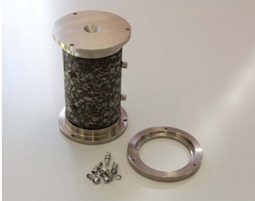
Figure 2.13: AMPT direct tension fatigue test specimen and end caps (end caps glued to specimen).
