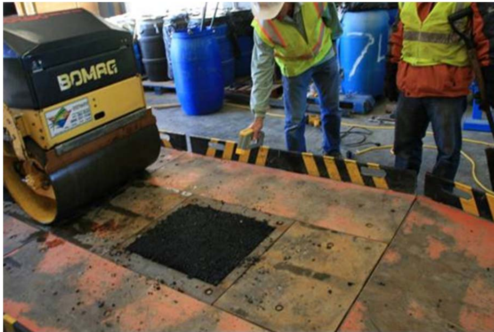
Figure 2.24: HMA specimen production by rolling-wheel compaction.
