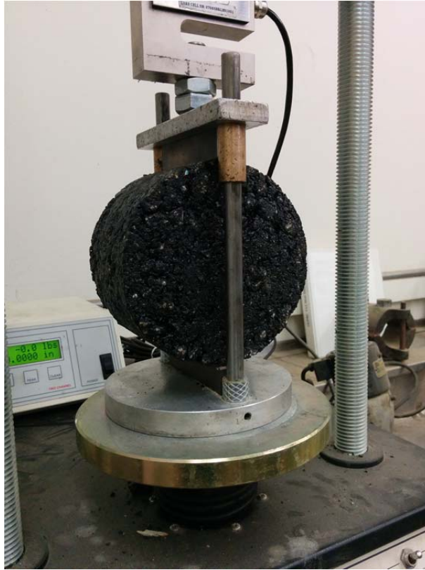
Figure 2.18 Indirect Tensile Strength (IDT) test device and specimen.
