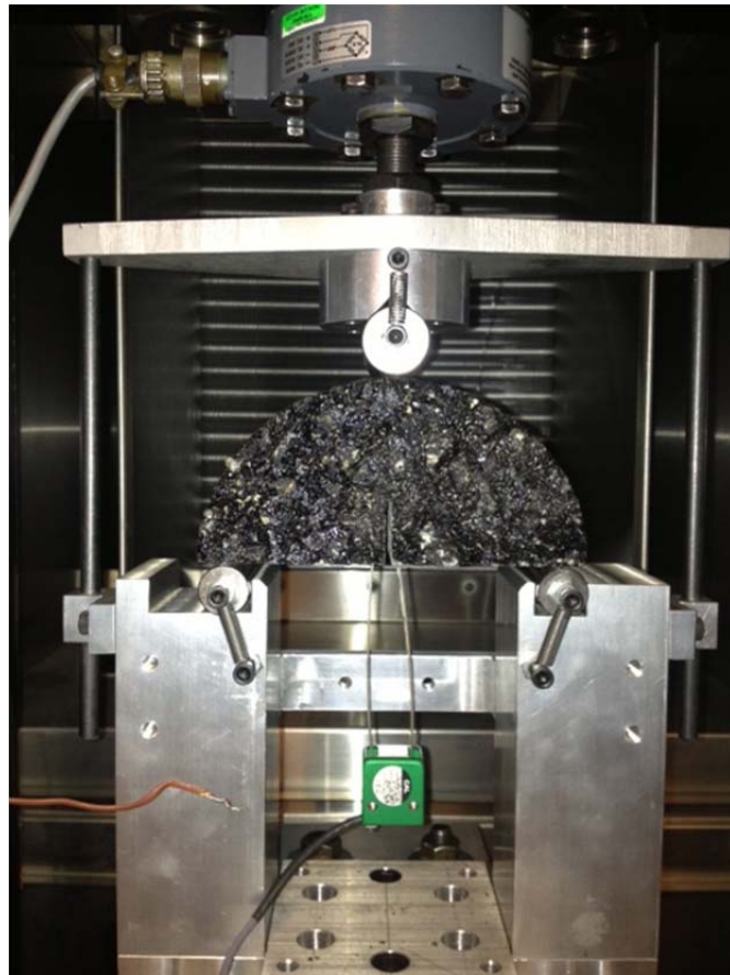
Figure 2.20: SCB test apparatus with specimen under test.
