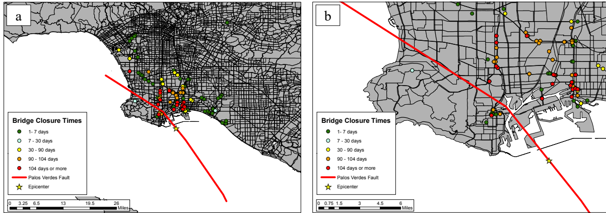
Figure 4.6: The location of damaged bridges within the general study region (a), and along the rupture length color-coded in terms of downtimes (b)
