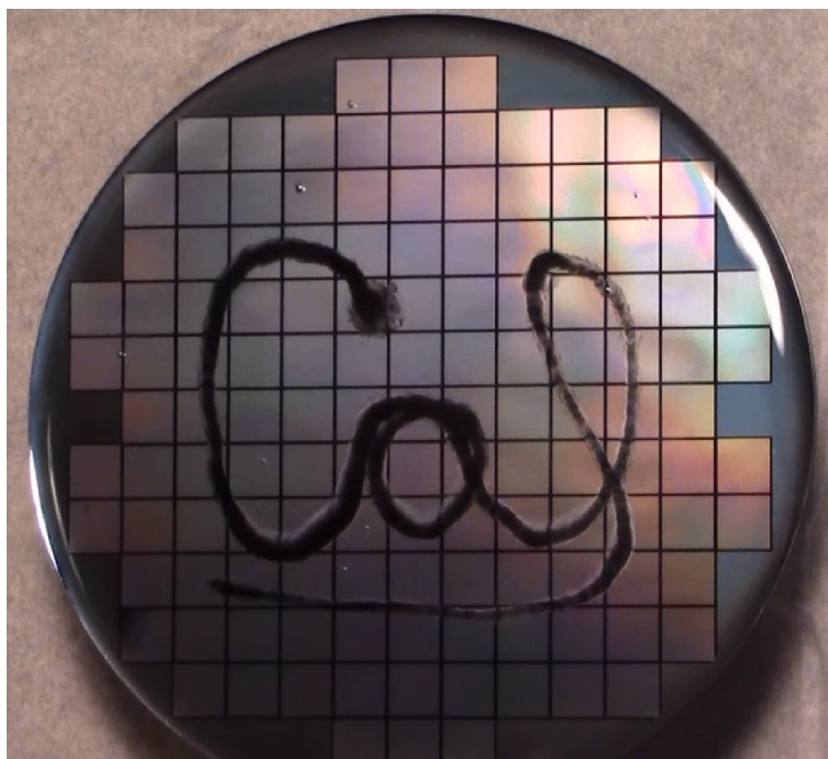
Figure 4.18: Wafer after dissolution of sacrificial germanium layer. Silica beads have been lifted off along the shape of a script 'Cal' delivered by a spray of deionized water.
