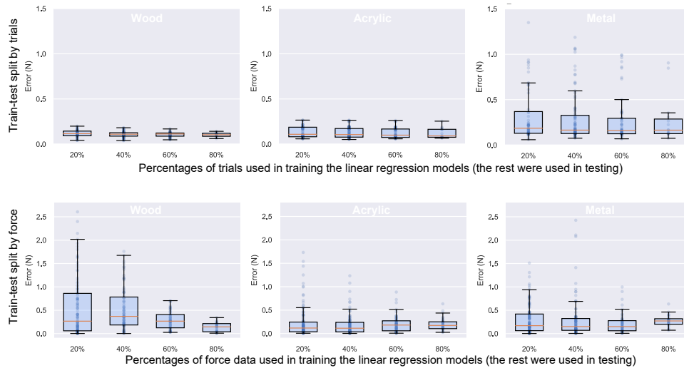
Figure 3.7: Evaluation results on sheets of three materials (wood, acrylic, metal) of various thicknesses.
