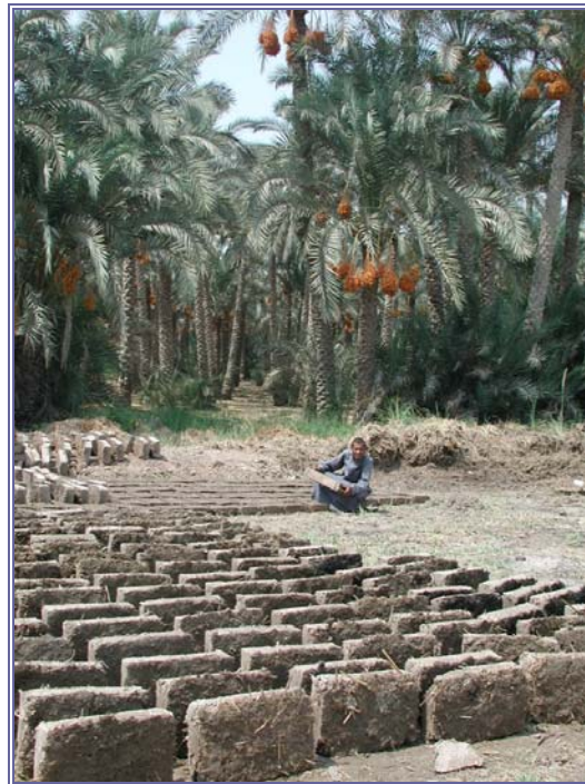
Figure 2. Striking new mud-brick. Note the earth-straw mixture in the background and brick turned for drying in the foreground.
