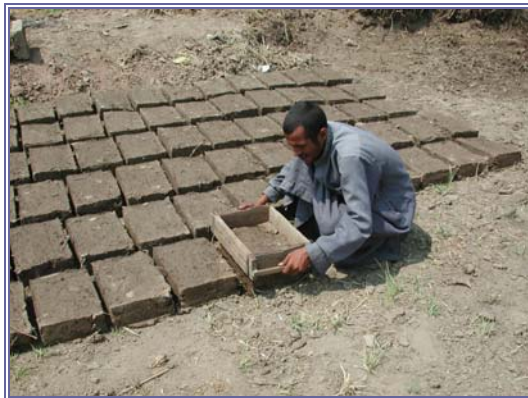
Figure 1. Unmolding new mud-brick.
