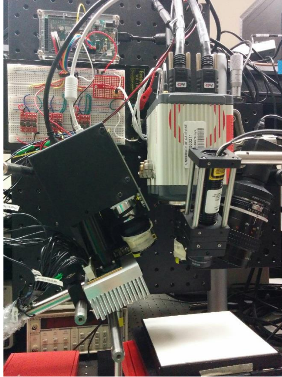
Figure 2.1 The high-speed SFDI and LSI instruments (Version 1)
