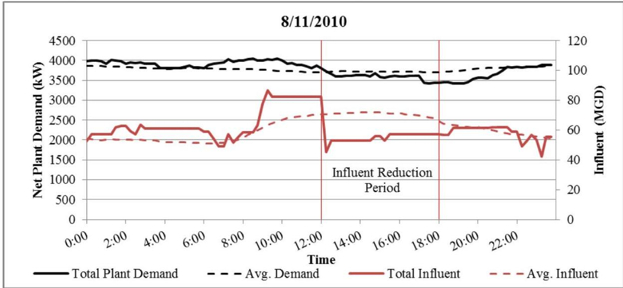
On the three days where flow from the North Shore Pumping Station was curtailed, demand from the pumping station was notably lower. On each day, demand was reduced by over 50% during the test period when compared to the dry season average, as seen in Figure 15.
