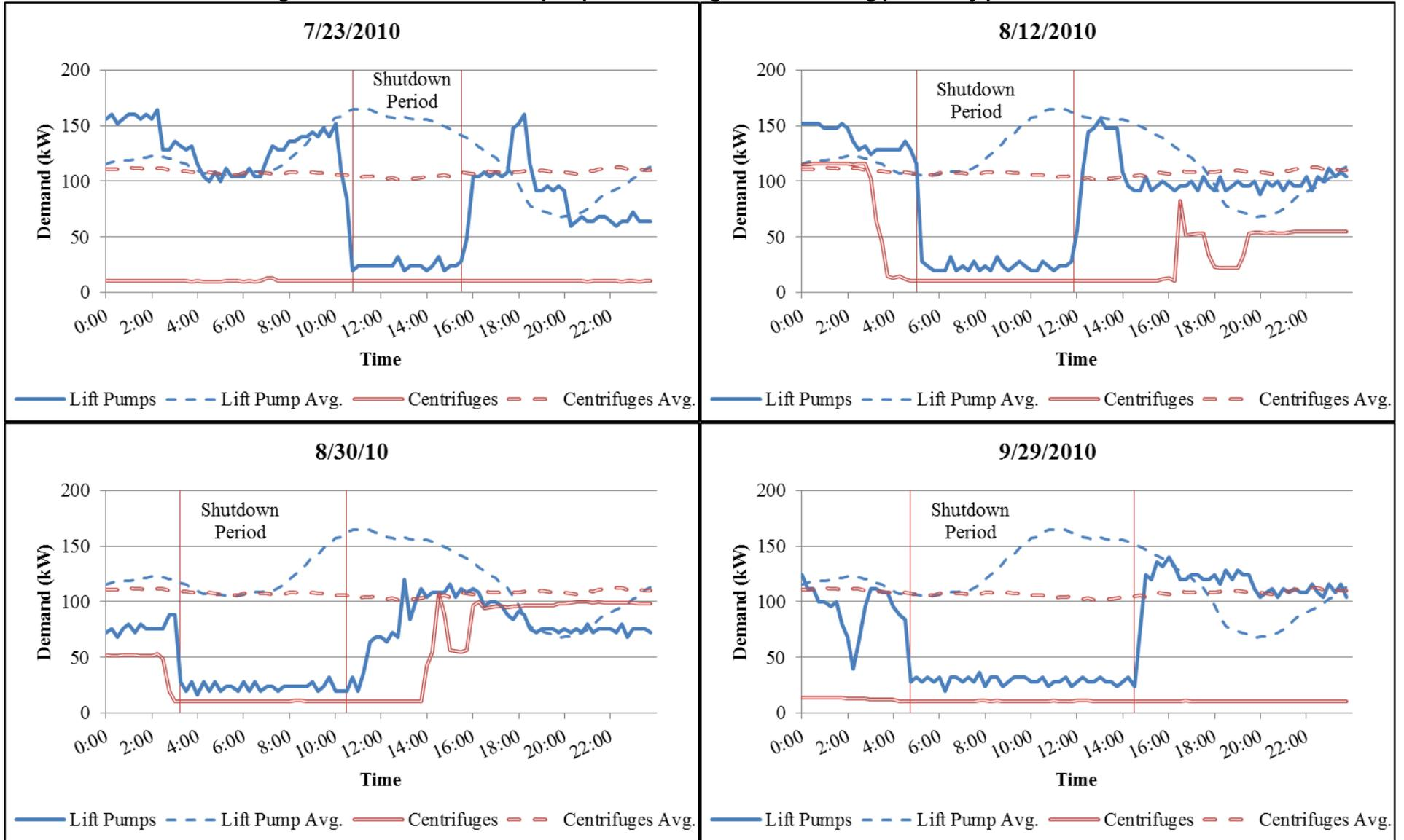
Figure A-16: Plant demand on flow adjustment days
