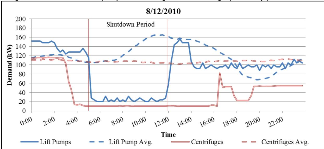
During the shutdowns, total centrifuge demand was reduced by 93-97 kW, an average of 90% of baseline dry season demand, as summarized in Table 8. As seen with the lift pumps, during each of the shutdowns where the centrifuges were active before the event, the total demand ramped down rapidly, fast enough to completely transition from normal operation to standby in less than an hour.
