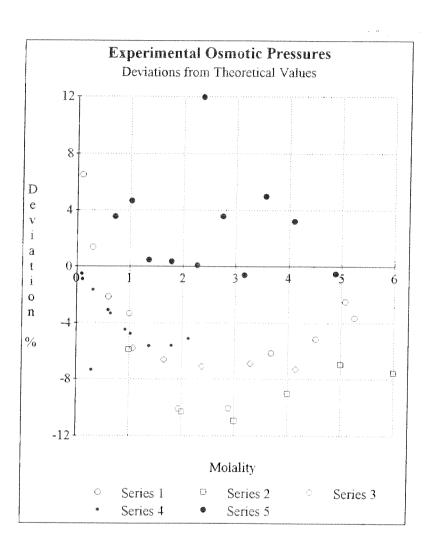
**Figure 6.** Osmotic pressures of aqueous solutions of sucrose. Deviations of experimental data from theoretical values by the present theory
