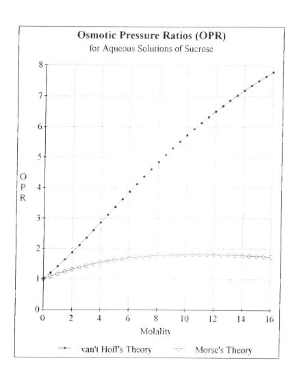
**Figure 4.** Osmotic pressures of aqueous solutions of sucrose. Comparison of the present theory with the classical theories of van't Hoff and Morse
