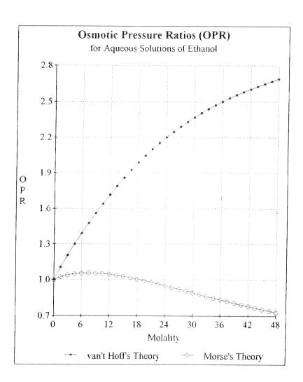
Figure 3. Osmotic pressures of aqueous solutions of ethanol. Comparison of the present theory with the classical theories of van't Hoff and Morse
