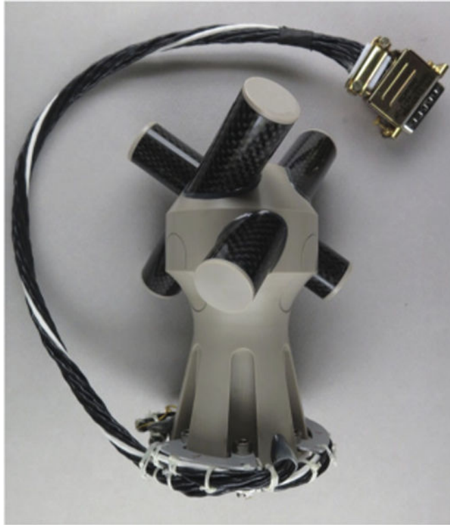
Fig. 11. Engineering model of the search-coil magnetometer (SCM) for SPP
