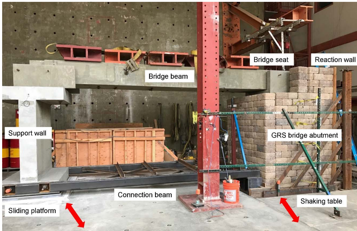
Figure 1. Configuration of GRS bridge abutment system (shaking direction indicated by red arrows).
